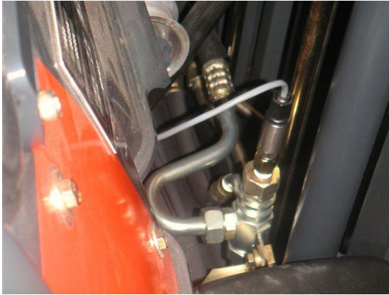
Typical Installation of the ED2 Series Pressure Transducer in Lifting Hydraulic Circuit
