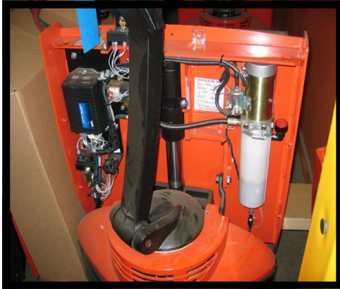
Typical Installation of the ED2-EPT Series Pressure Transducer in Lifting Hydraulic Circuit
