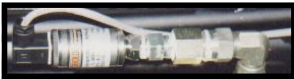
Typical Installation of the ED2-EPT Series Pressure Transducer in Lifting Hydraulic Circuit
