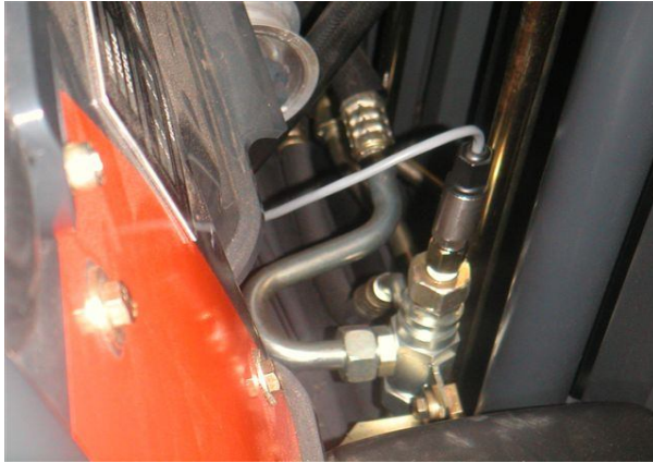
Typical Installation of the ED2 Series Pressure Transducer in Lifting Hydraulic Circuit
